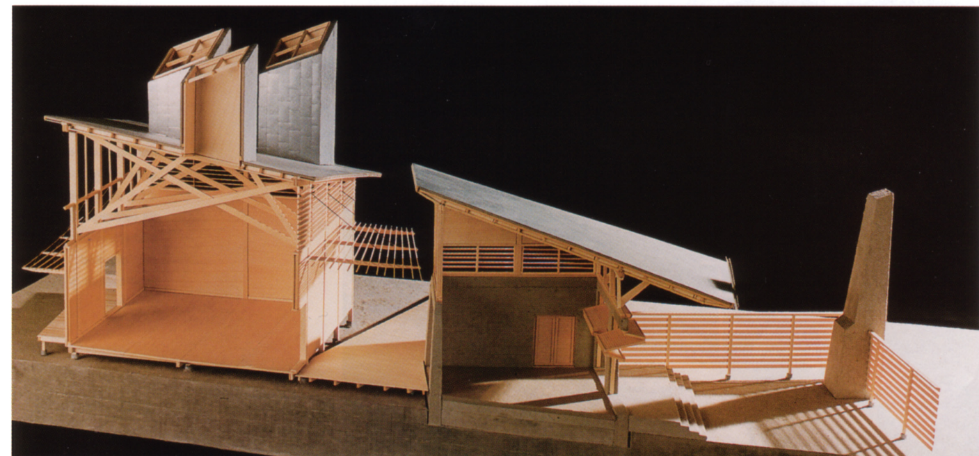
A sectional model of the painting and sculpture studios shows what Rose calls the “structural exhibitionism” of wood trusses.
